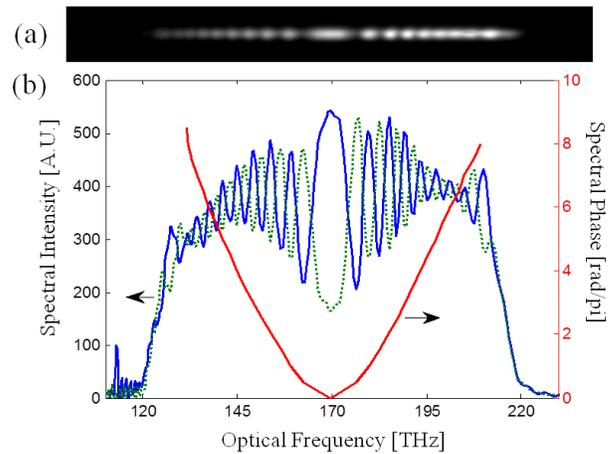
FIG. 3: (color online) Spectral fringes (a) normalized CCD image of the spectral fringes after both crystals. (b) Two calibrated fringe spectra with a  $\pi$  phase shift between them (blue and dotted green lines); and the corresponding calculated spectral phase  $\Phi(\omega)/2$  of the bi-photons (red line).
