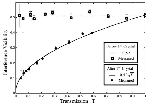
FIG. 4: Measured interference visibility as function of attenuation with corresponding theoretical fits before the first crystal (squares + dotted fit) and between crystals (circles + solid fit).
