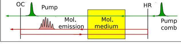
FIG. 1: The conceptual operation of the apparatus, where the pump pulse is followed by a coherent stimulated emission due to interaction with the recurring accumulated emission from previous pulses.
